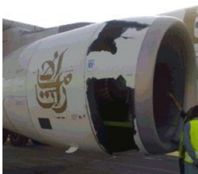
FIGURE 4: Engine Cowling Damage FAA States “Non-Hazardous Engine Effects”
