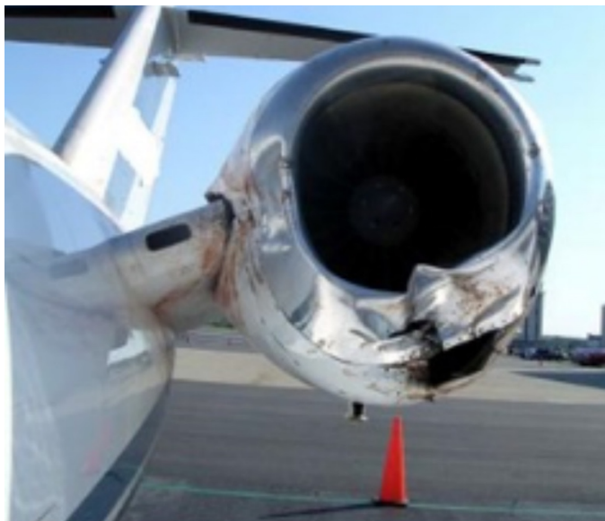
FIGURE 1: Engine Inlet Damage FAA States “Non-Hazardous Engine Effects”
