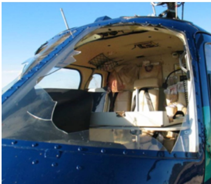
FIGURE 3: Helicopter Windshield Damage FAA States “Non-Dangerous Fragments”
