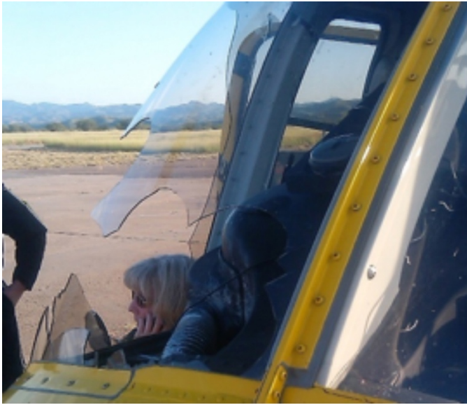
FIGURE 5: Bell 407 Windshield Damage FAA States “Non-Dangerous Fragments” (BirdStrike Consulting & Training)
