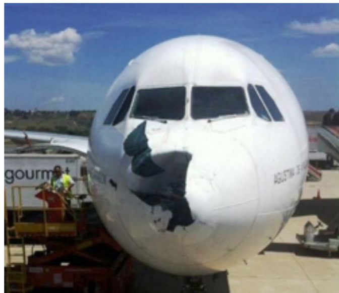
FIGURE 2: Nose Cone Damage FAA States “Safe Flight/Safe Landing”
