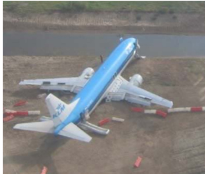
FIGURE 6: KLM PH-BTC Nose Gear Failure at Landing, Aircraft Total Loss (FS Passengers, 2008)
